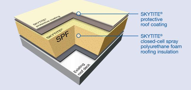
BASF offers SKYTITE<sup>®</sup> high-performance, spray-applied polyurethane foam (SPF) roofing systems for improved building durability and energy efficiency, coupled with the lowest lifecycle cost.
