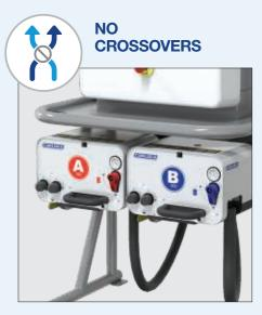
Independent, metered A & B materials reduce the risk of crossovers in the ST-1 Gun. The system will automatically shut down if it detects excessive flow of one material over the other.
